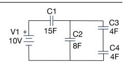
**Answer:** (C) 6 F. The two 4F capacitors in series reduce to 2F; added to the 8F capacitor in parallel gives 10F; 10F & 15F in series gives a total equivalent capacitance of 6F.
