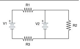
**Answers:** (B) & (C). The potential across  $R_2$  is completely controlled by  $V_2$ . Therefore, to increase the current across  $R_2$ , you can either increase  $V_2$  or decrease the resistance of  $R_2$ .
